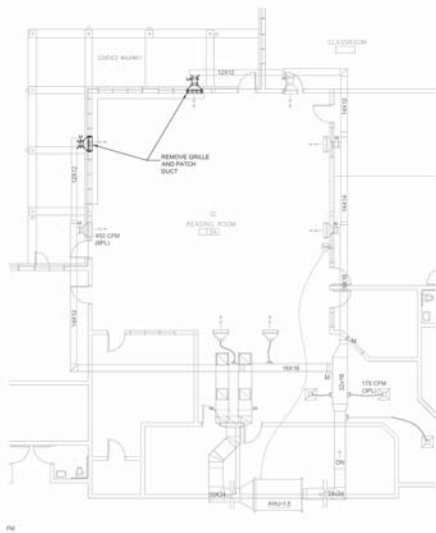
3.1 1 BUILDING 1 MEDIA CENTER AREA - DEMOLITION PLAN SCALE 1/8" = 1'-0"
