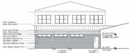
4 BUILDING 01 MEDIA CENTER ELEVATION SCALE 1/8"=1'-0"
