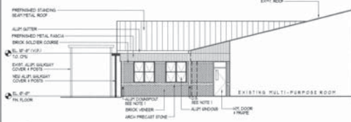
3 BUILDING 01 MUTIPURPOSE ELEVATION SCALE 1/8"=1'-0"
